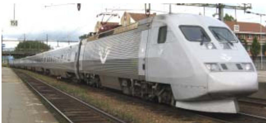
Figure 2 X 2000 high-speed tilting train, operated by SJ AB
