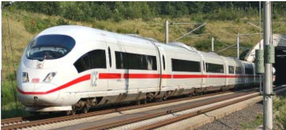
Figure 8 The ICE3 train, designed for a maximum speed of 330 km/h
