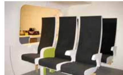
Test model of foldable and adjustable head rest
