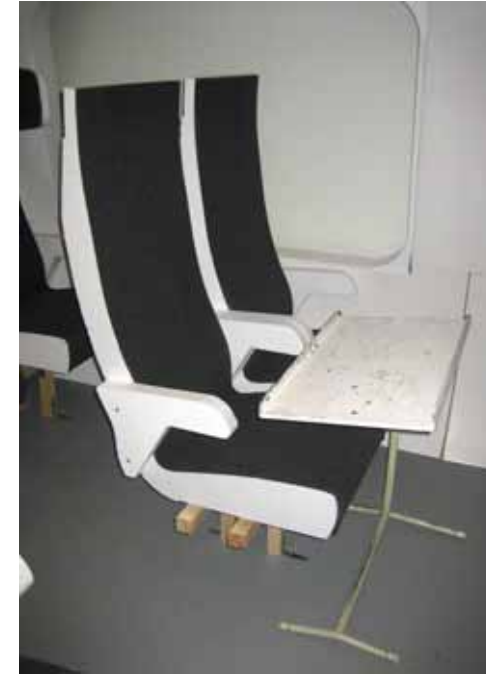
Test model of table placed on your own seat
