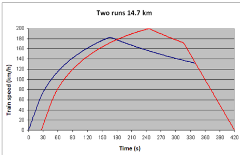
Figure 22. The train with eco-driving system (blue line) uses a time margin and starts earlier. Train not using the system (red line) has to drive faster to reach the destination at the same time. (Figure - Courtesy of Bombardier Transportation)
