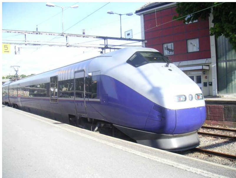
Figure 7-1: The Norwegian tilting train, class BM73, used in the Nordic field test by FACT, [Förstberg et al. 2005].
