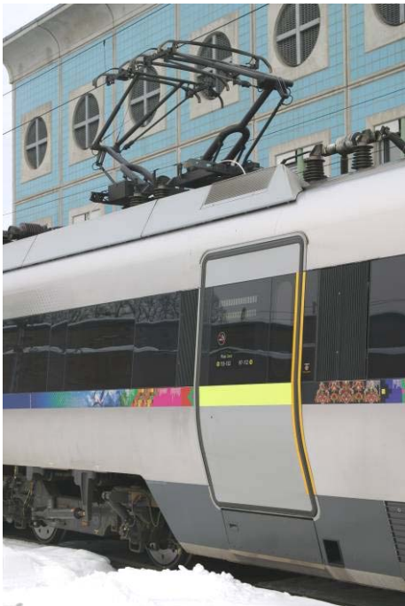
Figure 22. Above: High positioned air intakes on the Finnish Sm3.
