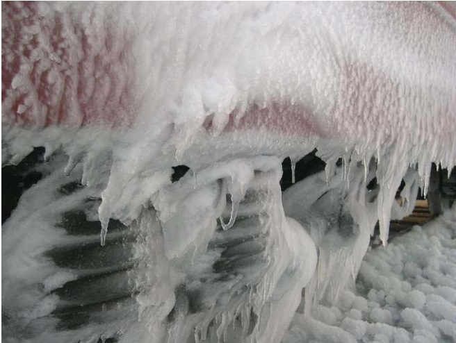
Figure 12. Bogie and carbody covered with ice.
