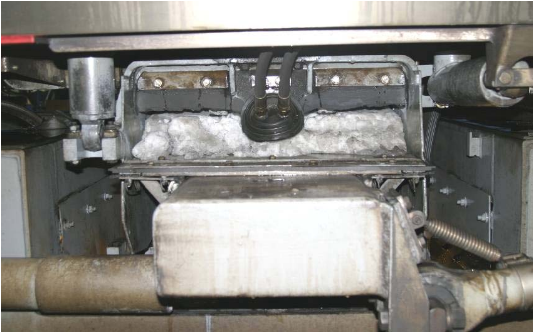
Figure 15. A rubber seal is mounted to prevent the snow to come further into the tilt mechanism.
