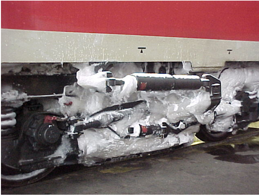
Figure 2. An example of a bogie with adhering ice.
