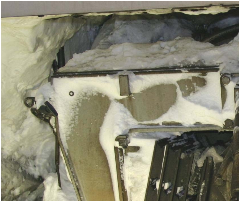
Figure 6. The thin plexiglass layer can be seen on the top of the bogie frame of a Swedish X2 trainset. The primary rubber suspension can be seen below to the right.
