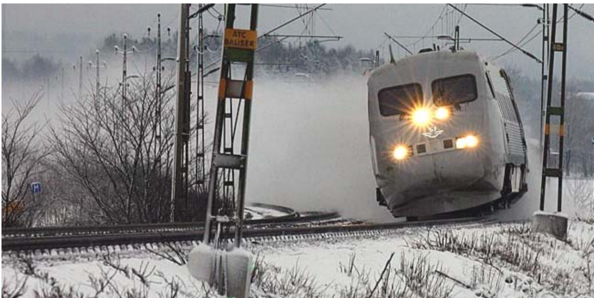
Figure 1. Snow smoke from the Swedish X2 trainset. Although the track seems more or less free from snow, the train is surrounded by a cloud of snow.
