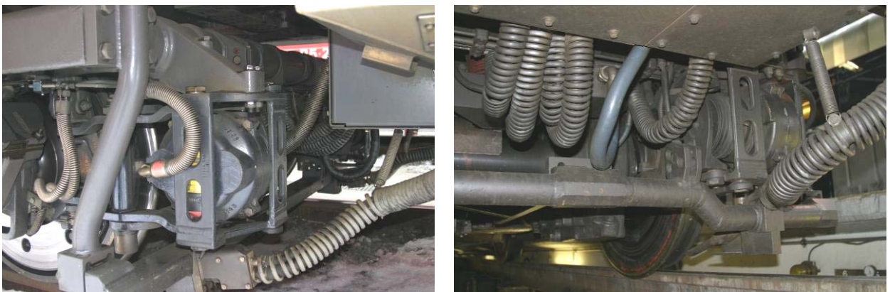
Figure 21. Cable protection devices on the Norwegian BM 71.
