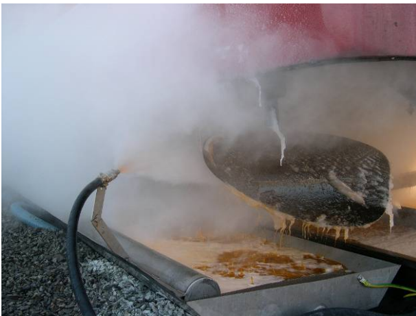
Figure 25. De-icing with propylene glycol in Drammen, Norway.
