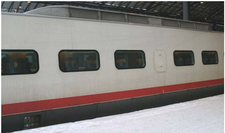
Figure 22. Above: High positioned air intakes on the Finnish Sm3.
