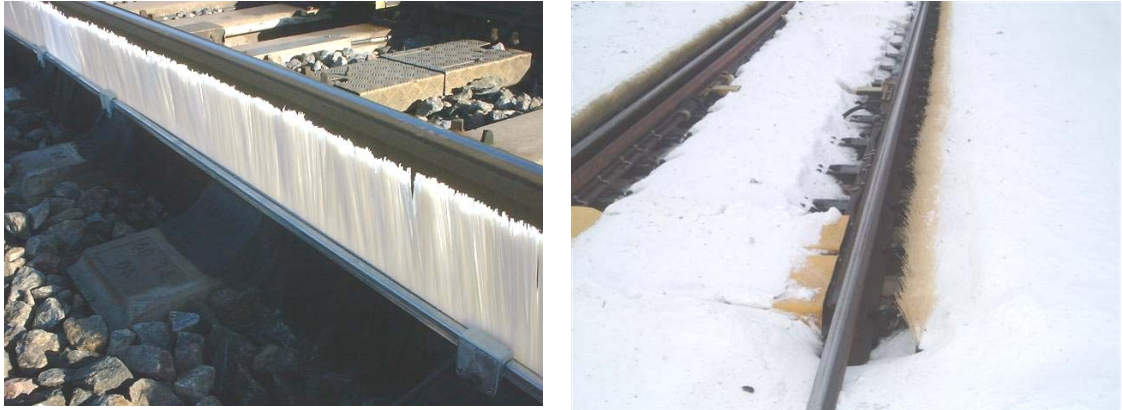
Figure 32. Detail of a brush spoiler is seen to the left. To the right the mounting outside the main rails in a switch is shown.
