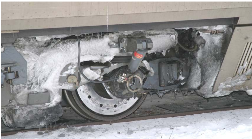
Figure 9. Snow and ice gatherings in a bogie, in the beginning of the ice build-up.
