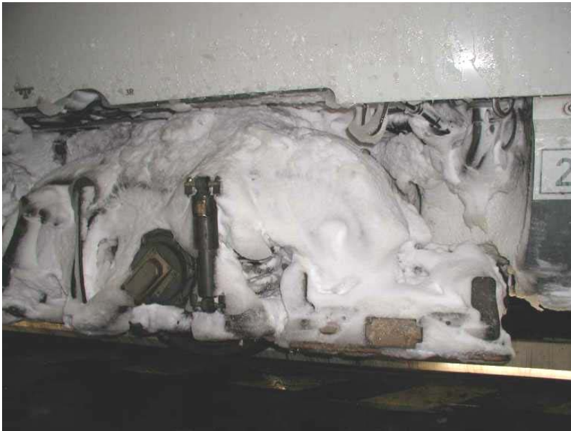
Figure 10. Snow and ice gatherings in a bogie after some time of operation.
